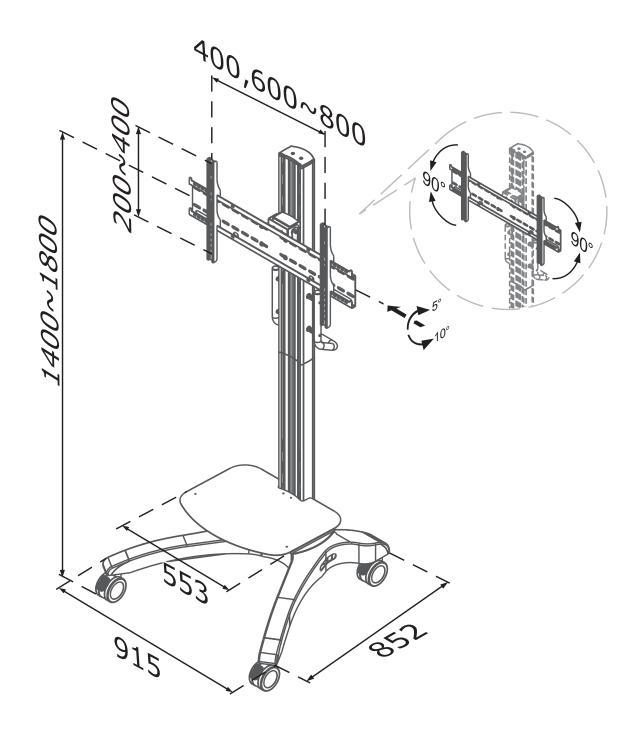
Neomounts Measuring unit: mm
